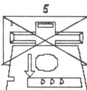
Drive 1 has failed Test 5. Remove the Digital Diagnostic Diskette (DDD) from the drive. The number above the drive tells which test is running.
