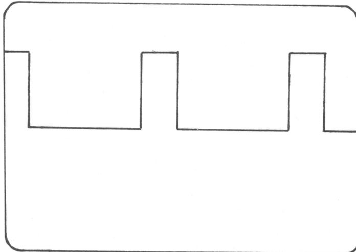
16. If necessary, adjust potentiometer R28 on the analog card until there is a single, stable image with a minimum of jitter.
