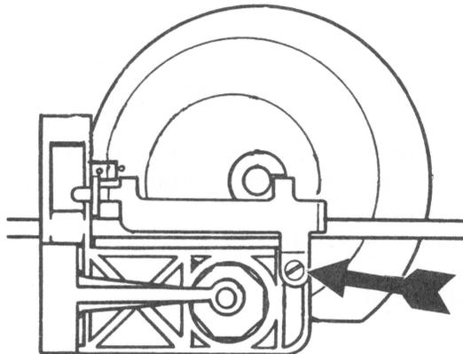
13. Move the carriage forward by hand until you feel the cam rider drop back into the channel of the cam.
