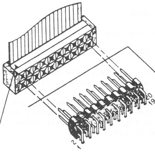
ARROW SHOULD BE UP WHEN CONNECTOR IS INSTALLED.
