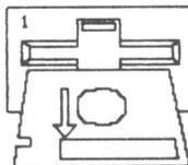
Remove non-write-protected, formatted diskette. (Arrow pointing away from drive means "Remove the diskette".)
