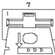
Drive 1 has passed Test 7 (and all previous tests). Remove the Digital Diagnostic Diskette (DDD) from the drive. (The DAP is finished and the drive has passed.)
