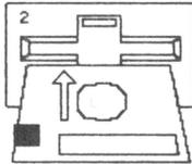
Insert write-protected, formatted diskette. (Arrow pointing toward drive means "Insert the diskette".)
