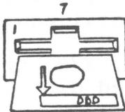
Drive 1 has passed Test 7 (and all previous tests). Remove the Digital Diagnostic Diskette (DDD) from the drive. (The DAP is finished and the drive has passed.)
