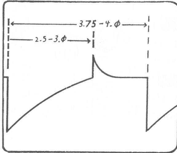
14. If necessary, adjust potentiometer R21 or R33 until the central peak is in the correct position.
