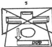
Drive 1 has failed Test 5. Remove the Digital Diagnostic Diskette (DDD) from the drive. The number above the drive tells which test is running.
